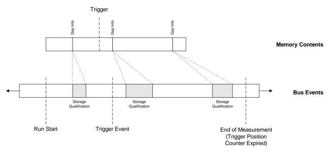
The following figure shows how the trace memory is filled.
