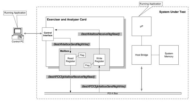
Programming Steps for Access via PCI-X Bus
