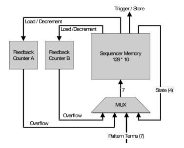
All sequencers provide an internal memory, state machine, and two 32-bit feedback counters (A and B). The statemachine controls the operation of the sequencer. The sequencer has 7 input registers. These registers can be used for input from pattern terms and for state feedback from the sequencer output. A maximum of  $2^4$ = 16 states is the practical limit—because at least one pattern term is always needed.
