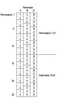
Furthermore, some values are not combined with all other values: for example, there is no tuple containing "1" and "C", and "2" is never combined with "D". The reason is that the repetition lengths of parameters A and D have a common factor (2).
