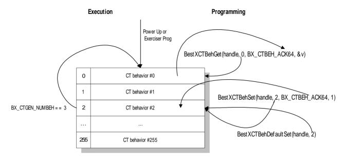
The following figure shows the memory design, the available functions to program the completer-target behavior memory, and the execution order.
